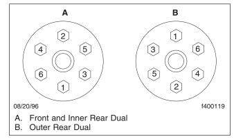
Fig. 1, Wheel Nut Tightening Sequence (6-stud hubs)
