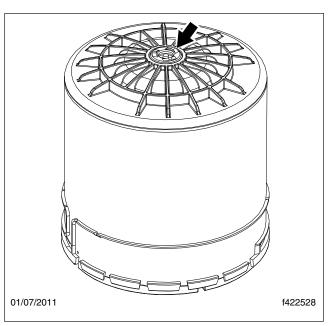
Fig. 3, New Cartridge with Rubber Spring
