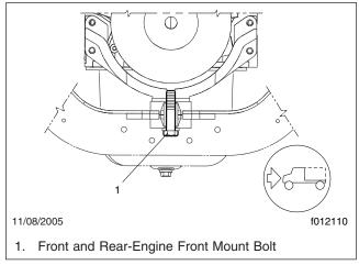
Fig. 2, Front and Rear-Engine Front Mount (ISB chassis built after 2002)
