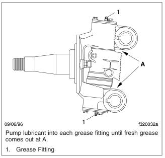
Fig. 3, Meritor Axle Grease Fittings
