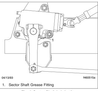
Fig. 4, Sector Shaft Lubricating
