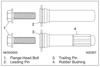
Fig. 9, ZOH-T Slide Pins and Bolts
