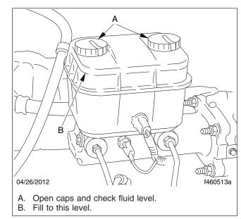
Fig. 8, Hydraulic Brake Fluid Reservoir
