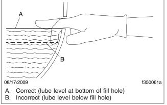
Fig. 3, Checking Axle Lubricant Level
