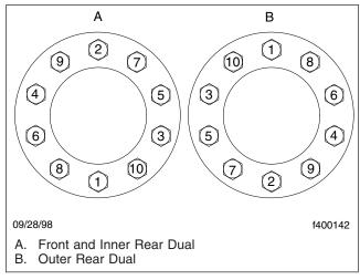
Fig. 3, Wheel Nut Tightening Sequence (10-stud hubs)
