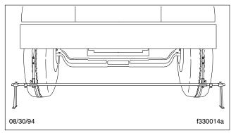
Fig. 7, Trammel Bar Positioning
