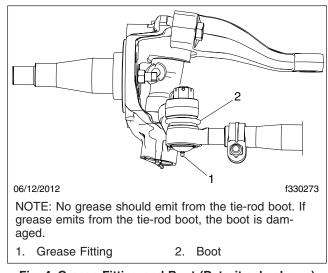
Fig. 4, Grease Fitting and Boot (Detroit axle shown)
