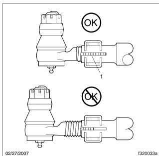
IMPORTANT: The tie-rod end threads must be visible throughout the entire length of the split.
