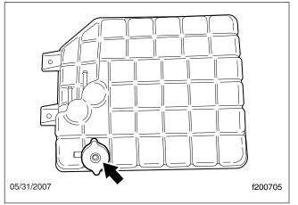
Fig. 1, Surge Tank Coolant Fill Cap
