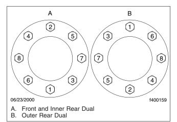
Fig. 2, Wheel Nut Tightening Sequence (8-stud hubs)
