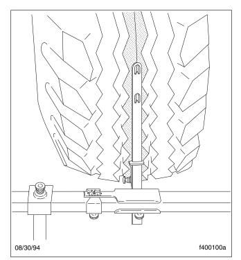
Fig. 8, Setting Trammel Bar Pointers
