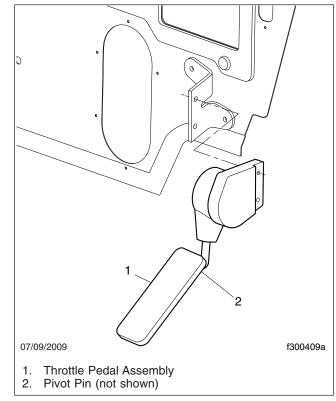
Fig. 2, Suspended Throttle Pedal
