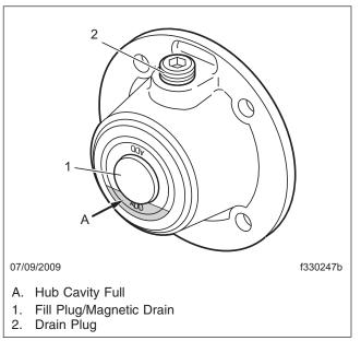
Fig. 11, Oil-Filled Hub Cap
