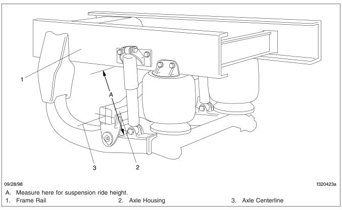
Fig. 1, Ride Height Inspection (typical Neway suspension shown)
