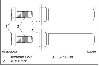
Fig. 10, ZOPS Slide Pins and Bolts
