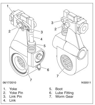
Fig. 7, Bendix Automatic Slack Adjuster
