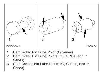
Fig. 11, Cam and Anchor Roller Pin Lubrication Points
