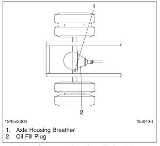
Fig. 2, Component Locations, Meritor Axles
