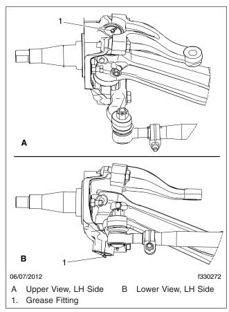
Fig. 1, Grease Fittings, Detroit Axles
