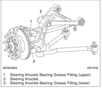
Fig. 4, Pressure Grease Fitting Positions, RL-75E
