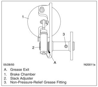
Fig. 5, Camshaft Bracket Bushing Lubrication
