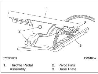
Fig. 1, Floor-Mounted Throttle Pedal
