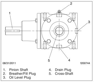
Fig. 2, Mechanical Fan Drive Gearbox
