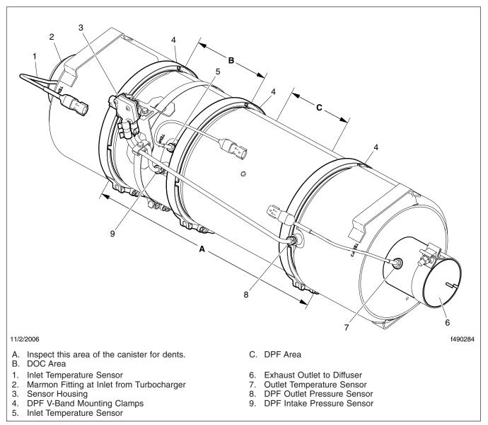
Fig. 2, Cummins Aftertreatment Device
