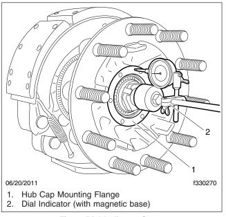
Fig. 9, Dial Indicator Setup
