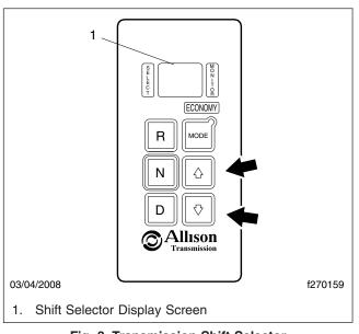
Fig. 3, Transmission Shift Selector
